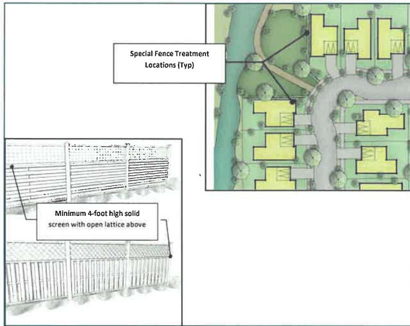
Figure 31: Fencing at Open Space
