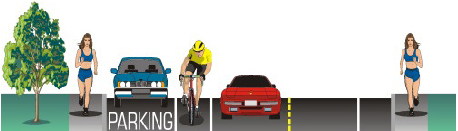
Figure 10: Class II Bikeway with On-Street Parking
