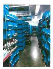
Remaining samples are stored at 4 degrees C in walk-in refrigerators. Temperatures in all cold storage areas are measured twice each day to ensure required temperature is maintained (NELAC 5.5.3). Volatiles samples are segregated in separate refrigerators to prevent cross-contamination.
