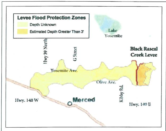
Levee Flood Protection Zones estimate the maximum area that may be inundated if a project levee fails when water surface elevation is at the top of a project levee. Zones depicted on this map were created utilizing methods and assumptions described in the accompanying technical manual, and do not necessarily depict areas likely to be protected from flow events for which project levees were designed.
